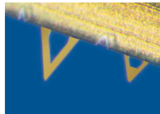
Both V- and A-shaped cantilevers have a large enough triangular area near the apex to ensure laser light reflection.
